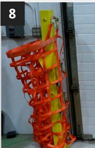
8. Stow by disconnecting from one side and rolling to the other. Hook the top strap to the top eyebolt as shown to the left.
