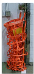
5. Stow by disconnecting from one side and rolling to the other. Hook the top strap to the top bracket as shown to the left.
